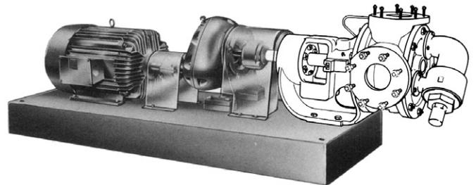
The large “C” size reducer also is available with two gear ratios, 6.24 to 1 and 7.95 to 1. It is normally used with the “Q” or “M” size pumps. Like the “A” and “B” reducers, the “C” reducer is bracket mounted and requires flexible couplings both for the input and output shafts. With the “C” reducer, “Q” and “M” size pumps, driven by 1200 RPM motors, can cover a capacity range to 160 GPM.
