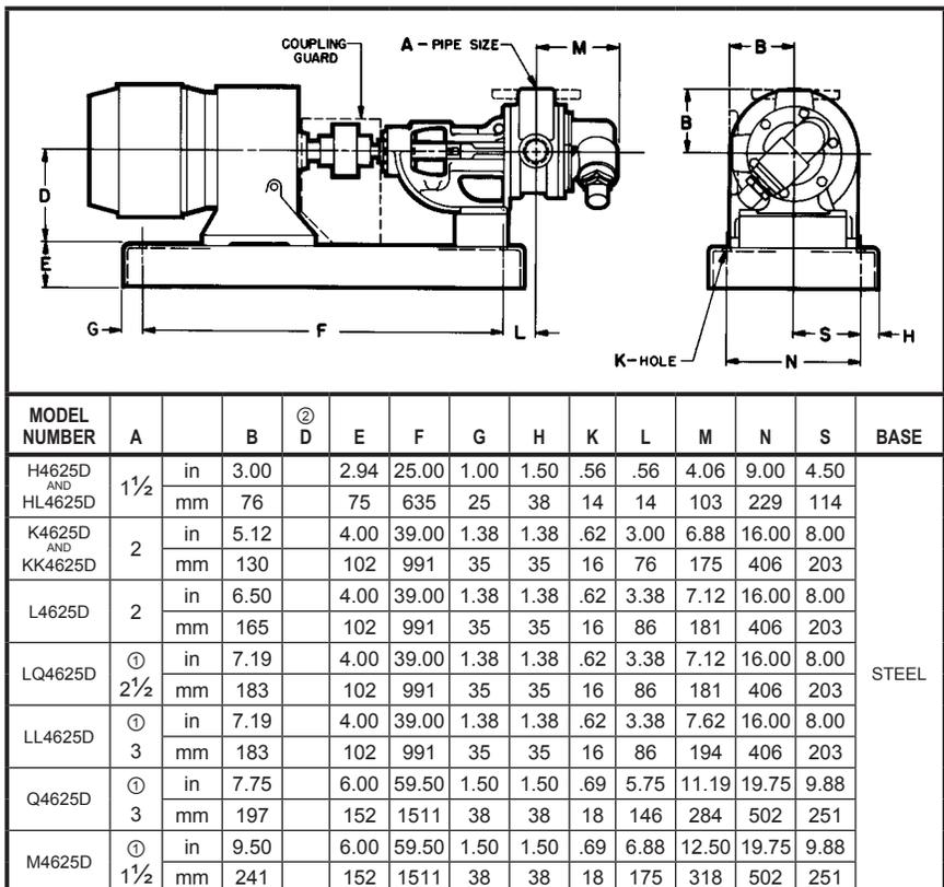
① Ports are suitable for use with 125# ANSI cast iron or 150# ANSI steel companion flanges or flanged fittings. All others tapped for standard pipe.
