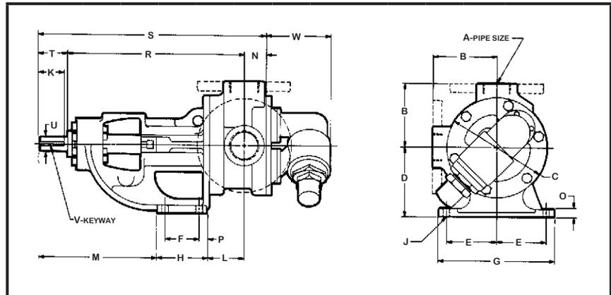
① Ports are suitable for use with 125# ANSI cast iron or 150# ANSI steel companion flanges or flanged fittings. All others tapped for standard pipe.
