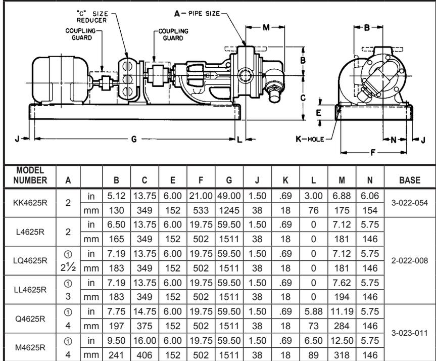
① Ports are suitable for use with 125# ANSI cast iron or 150# ANSI steel companion flanges or flanged fittings. All others tapped for standard pipe.
